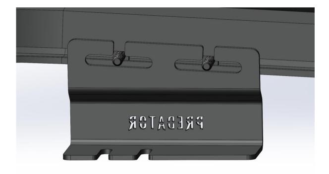
Once lowered, slide T-Slot bolts to either side of bracket and fit nuts (Don't fully tighten at this stage) Repeat for each mounting bracket.
