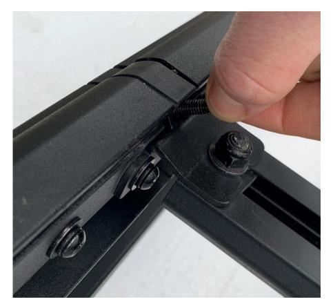
Slide T-slot bolts within the recessed channel to be roughly in position where mounting brackets will fix. This is -4 T-slots per side -2 towards the front on either side and 2 towards the rear on either side.
