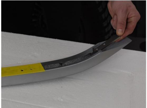
Place your forefinger through the acces hole in the top of roof rail, push fixing plate against bottom of rail & align threads so that fittings can be screwed through the 7mm holes and into the fixing plate. (Threadlocker advised on these fittings)
